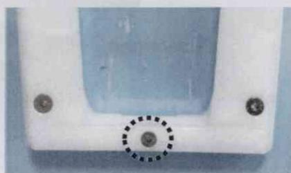
**Do not tighten too firmly the lower central bolt to ensure proper operation of the automatic locking mechanism**
